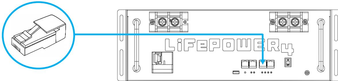
5. **Turn On Sequence:** Power on the master Model 3 battery first, then turn on each remaining Model 3 battery in order in ~5 second intervals. Once all Model 3 batteries are on, switch on the Model 2 batteries corresponding to their DIP switch number.
