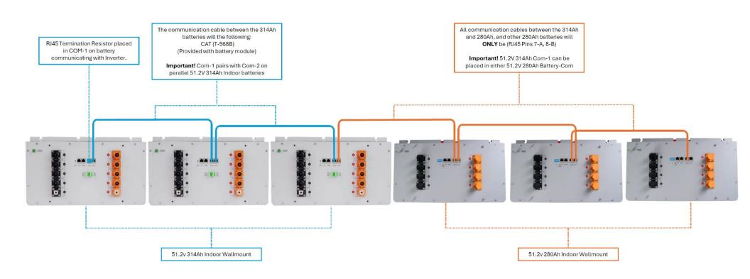
The photo above shows the proper connections for communication between multiple 314Ah and 280Ah batteries.
