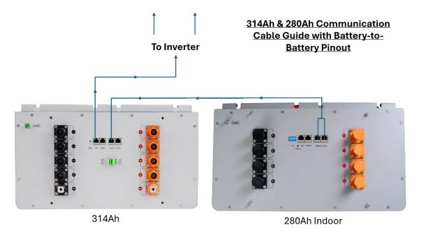
The photo above shows "Comm2" being used on the 314Ah, and either of the "Battery-Comms" being used on the 280Ah. Do not wire to both "Battery-Comms" ports, only one is required for the 314Ah battery, the other is used for daisy chaining to the next battery.
