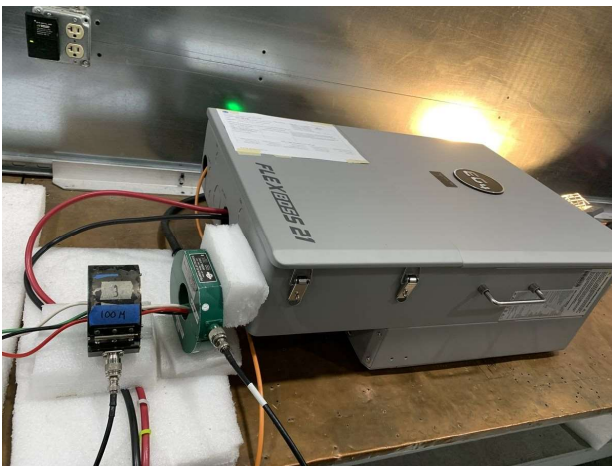
CS116 test on AC Full Bundle EMI#1
