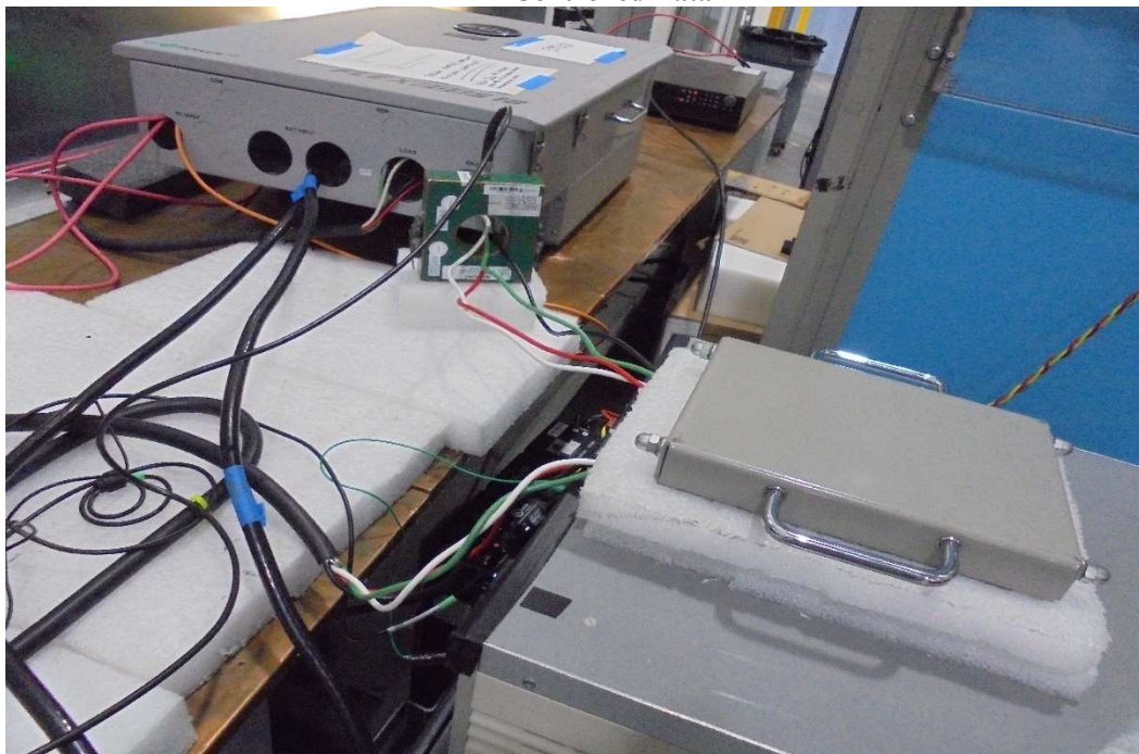
General Test Setup for CS117, Test Setup Waveform #1 – Actual Test on Full AC Bundle
