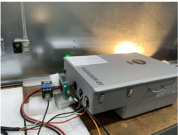
CS116 test on DC Bundle EMI#1
