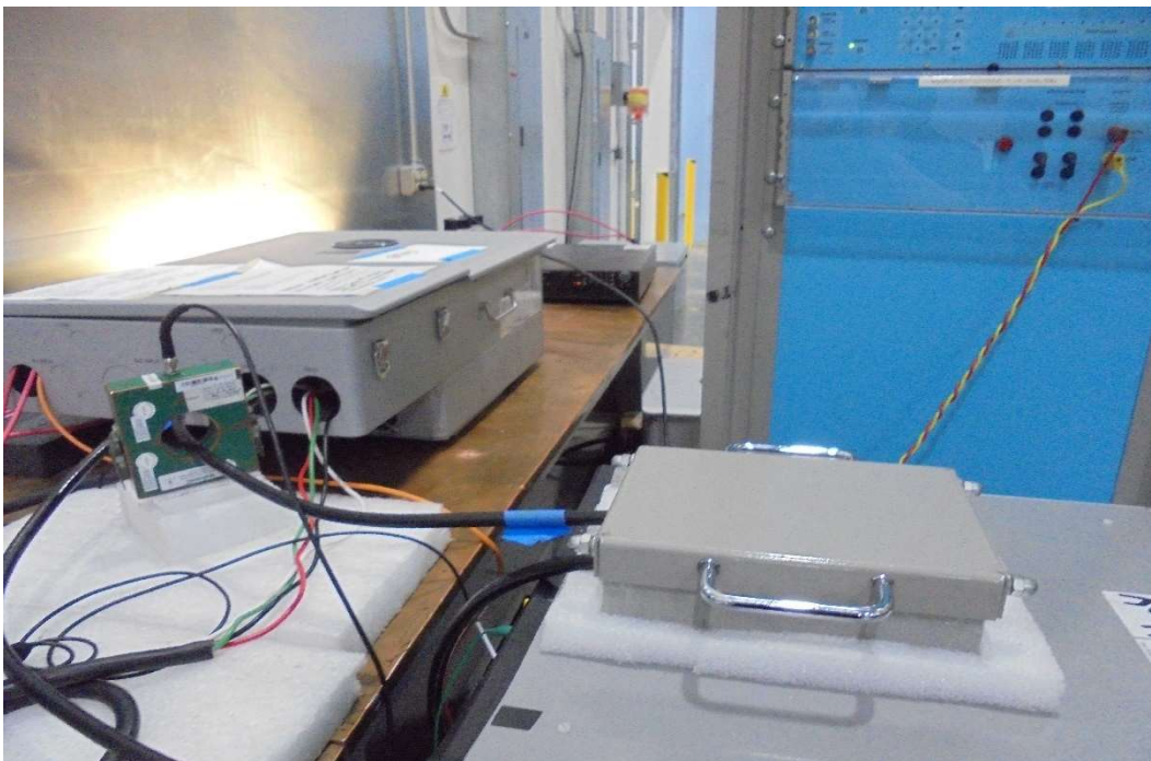
General Test Setup for CS117, Test Setup Waveform #1 – Actual Test on DC Return
