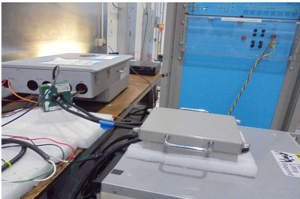
General Test Setup for CS117, Test Setup Waveform #1 – Actual Test on DC Power Bundle
