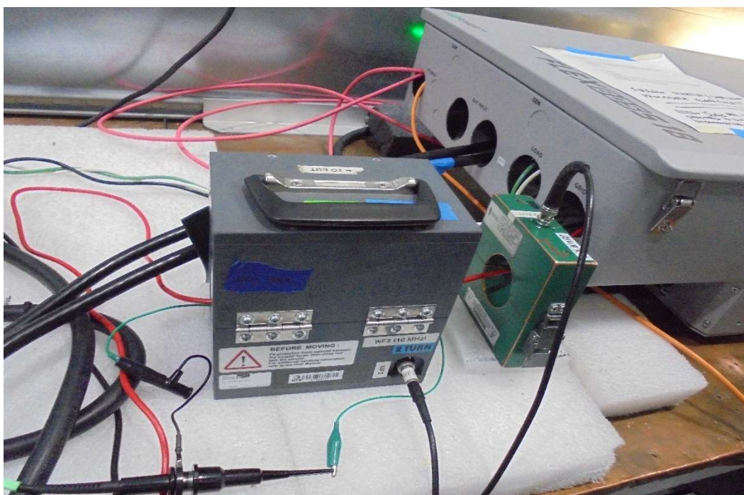
General Test Setup for CS117, Test Setup Waveform #2 & #3 – Actual Test on Line 1 AC Power
