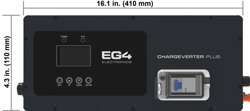
The EG4® Chargeverter Plus is a robust AC to DC converter designed specifically for 48 VDC lithium battery charging in on-grid and off-grid Energy Storage Systems. The charger can operate on 120, 208, or 240 VAC and is capable of up to 100A of DC charging current and IP-54 rated for outdoor installation.
