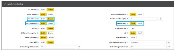
In this scenario by default, you will not be able to charge batteries with grid power, but we can change just a few settings to allow us to Grid Assist and charge the batteries with grid power. See the image below:
