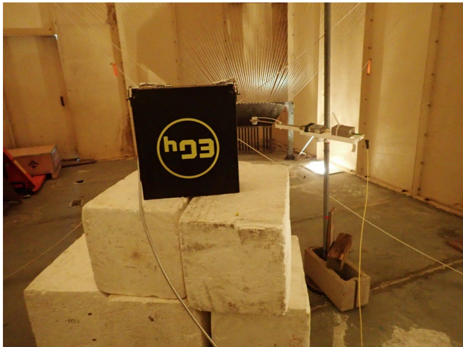
Test Setup of EG4 LL100Ah 48V Server Rack (Serial No. SC2022101794) on Z Axis
