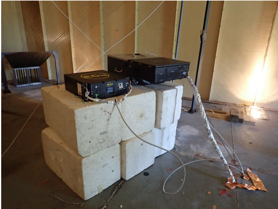
EG4 18kPV Hybrid Inverter (Serial No. 3464660222) with EG4 LL100Ah 48V Server Rack (Serial No. SC2022101794) on X Axis
