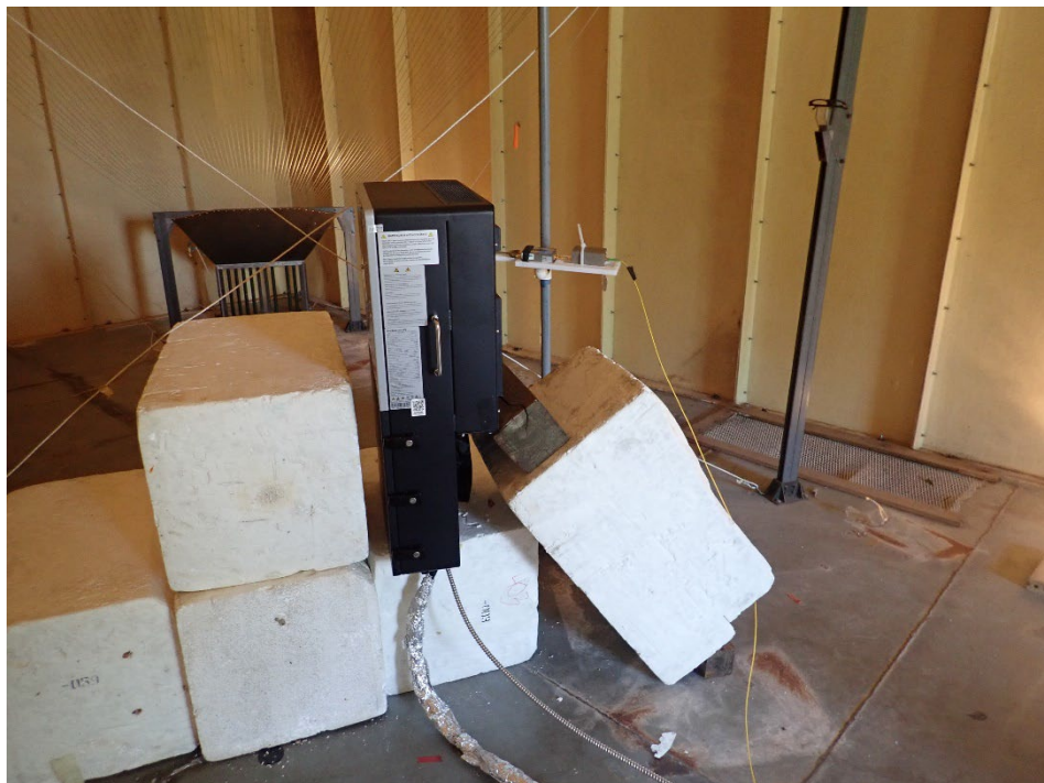
Test Setup of EG4 18kPV Hybrid Inverter (Serial No. 3464660222) on Z Axis
