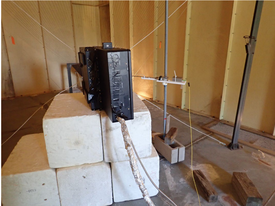
Test Setup of EG4 18kPV Hybrid Inverter (Serial No. 3464660222) on Y Axis
