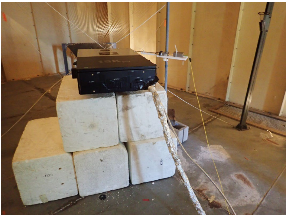
Test Setup of EG4 18kPV Hybrid Inverter (Serial No. 3464660222) on X Axis
