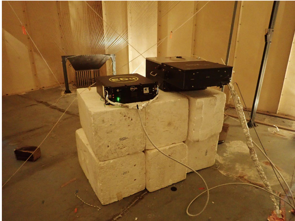
Test Setup of EG 4LL100Ah 48V Sever Rack (Serial No. SC2022101794) and EG4 18kPV Hybrid Inverter (Serial No. 3464660222) on X Axis
