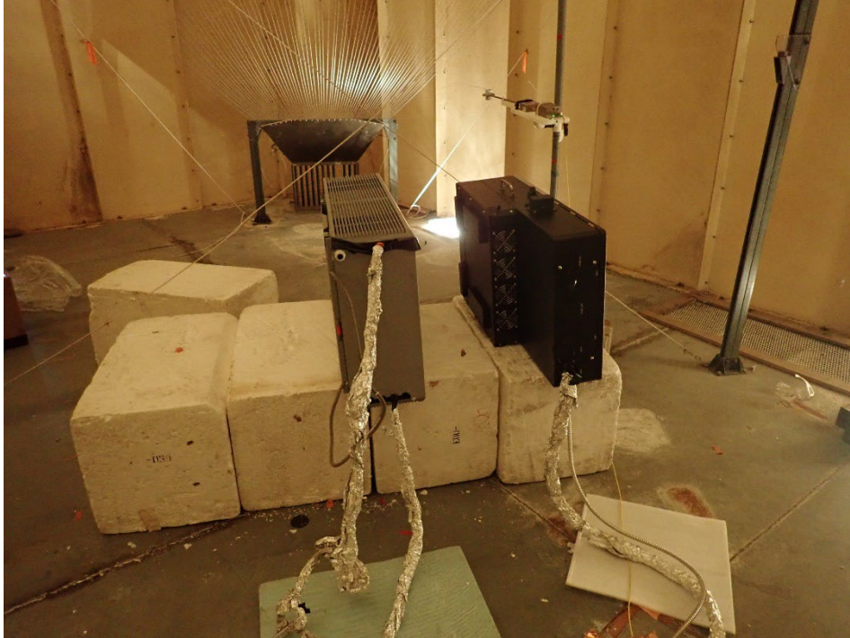
Test Setup of Unit EG4 18kPV Hybrid Inverter (Serial No. 3464660222) and EG4 LL280Ah 48V Wallmount (Serial No. SC2024010608) in Y Axis
