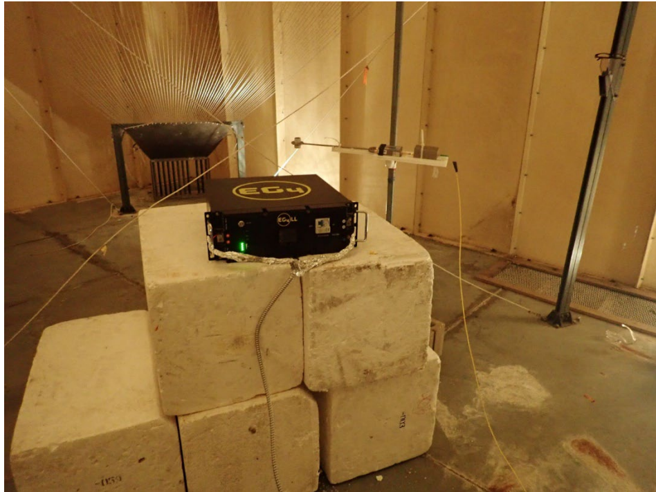
Test Setup of EG4 LL100Ah 48V Server Rack (Serial No. SC2022101794) on X Axis
