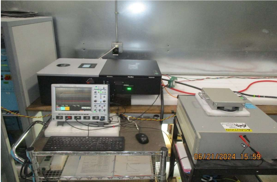
Test Setup for CS117, Actual Test Waveform #1 on Battery Return Side
