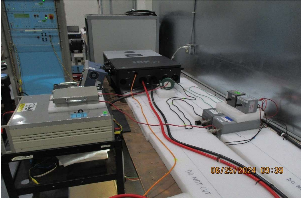
Test Setup for CS117, Actual Test Waveform #1 on AC Line 1
