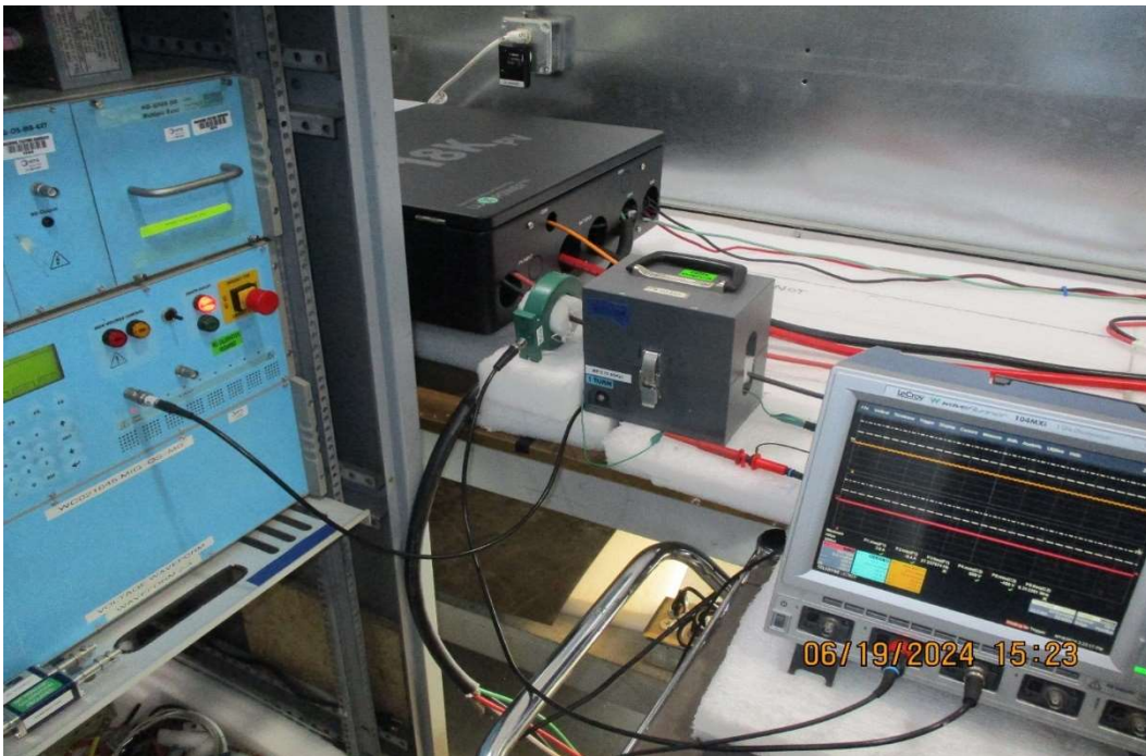
Test Setup for CS117, Actual Test Waveform #2 & #3 on PV Return Side
