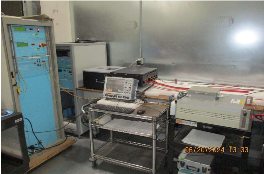
General Test Setup for CS117, General Test Setup for Waveform #1
