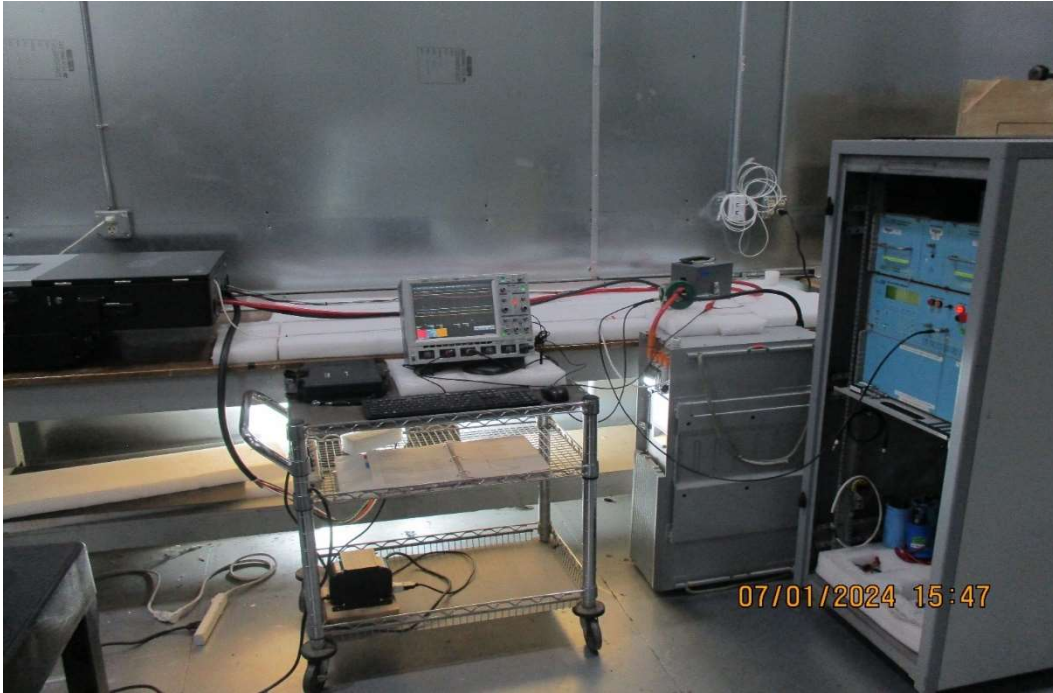
Test Setup for CS117, General Waveform #2 & #3 Test Setup for Battery Wall Mount
