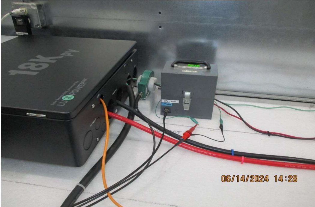
Test Setup for CS117, Actual Test Waveform #2 & #3 on AC Line 1
