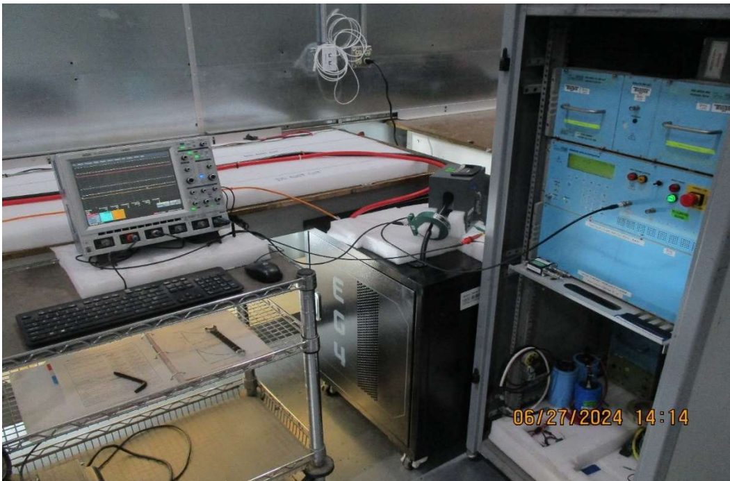
Test Setup for CS117, Actual Test Waveform #2 & #3 on Battery Return Side
