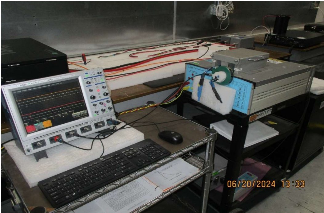
General Test Setup for CS117, General Test Setup for Waveform #1 – Open Circuit
