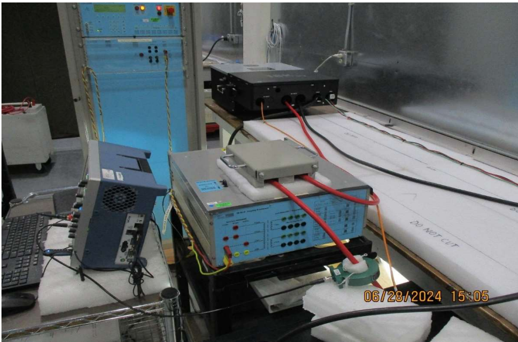
Test Setup for CS117, Actual Test Waveform #1 on Battery High Side
