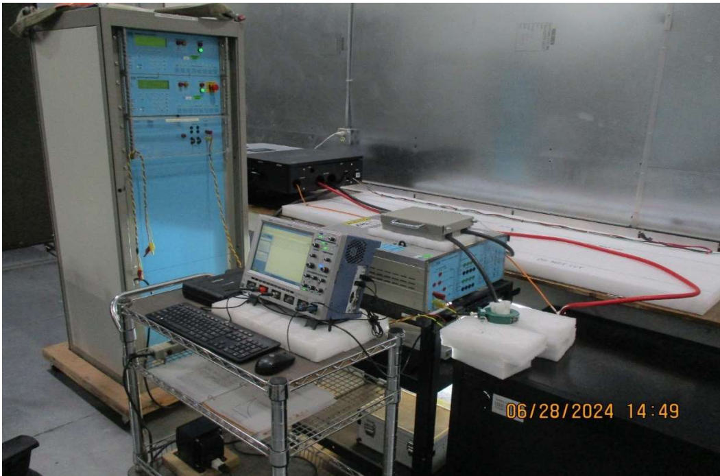
Test Setup for CS117, General Waveform #1 Test Setup for Battery Rack Mount
