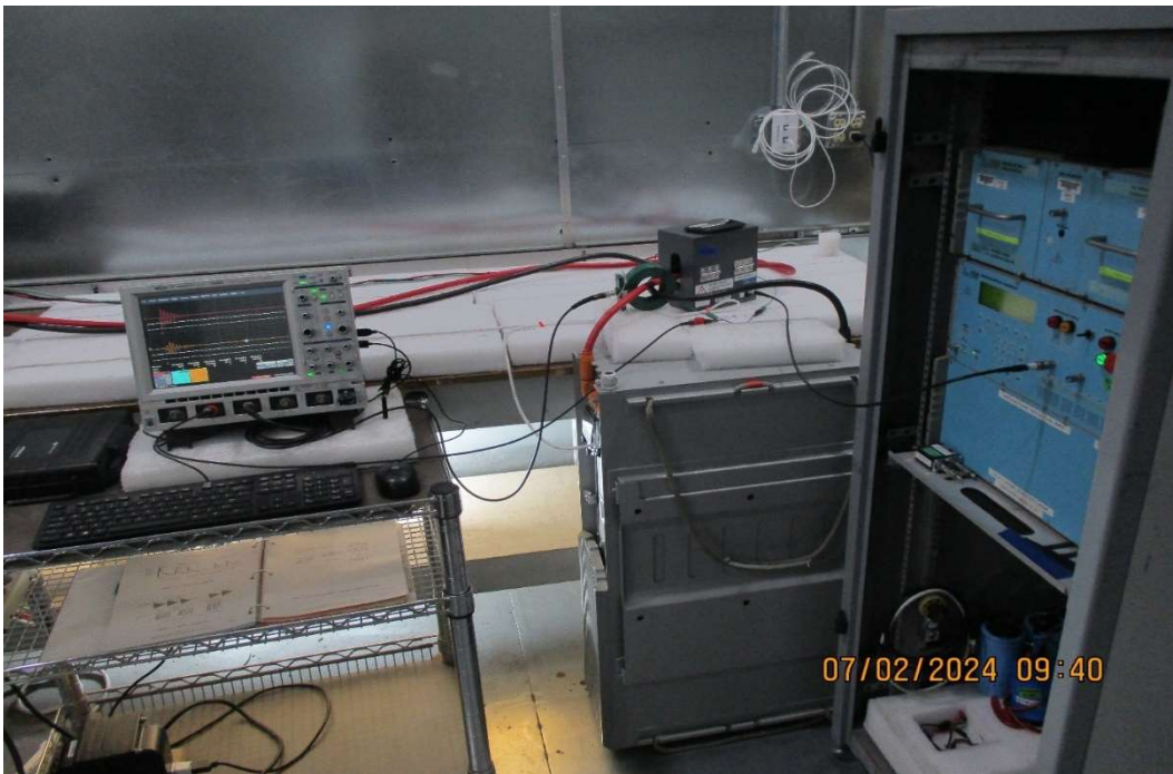
Test Setup for CS117, Actual Test Waveform #2 on Battery Bundle
