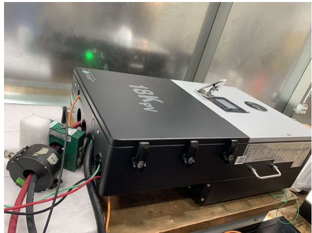
CS116 Test DC Bundle
