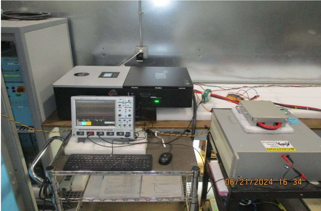
Test Setup for CS117, Actual Test Waveform #1 on Battery Bundle
