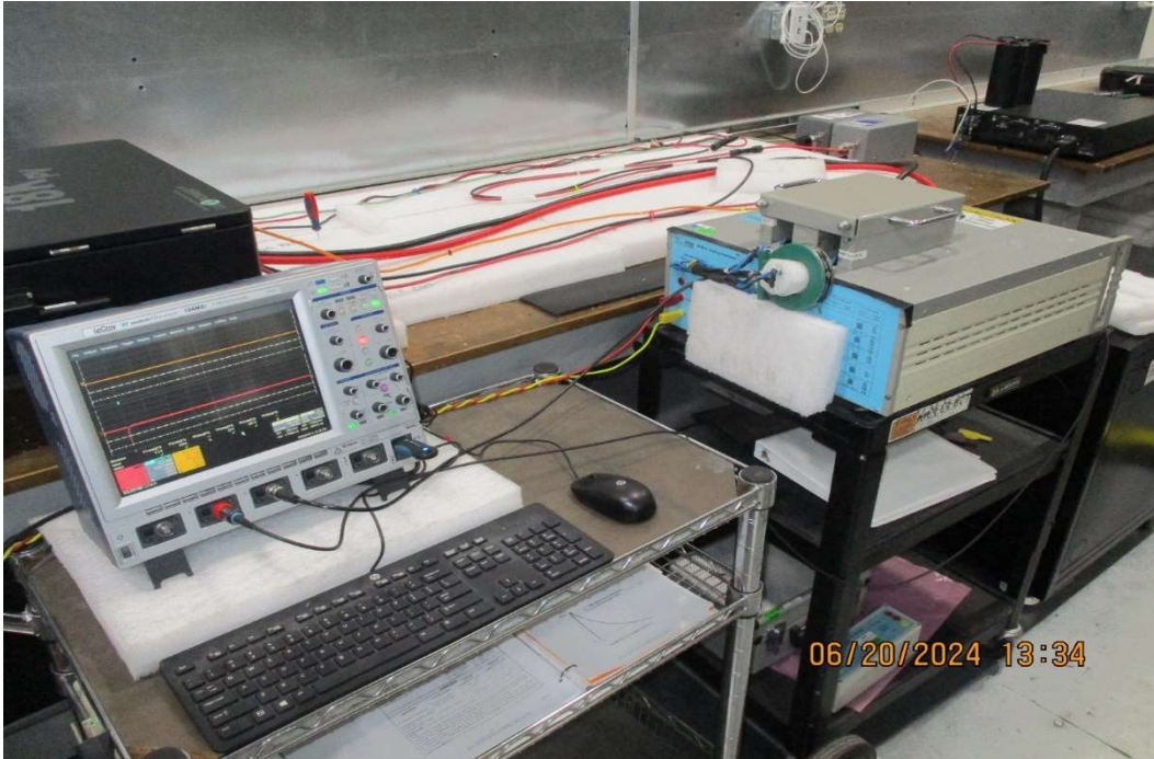
General Test Setup for CS117, General Test Setup for Waveform #1 – Short Circuit
