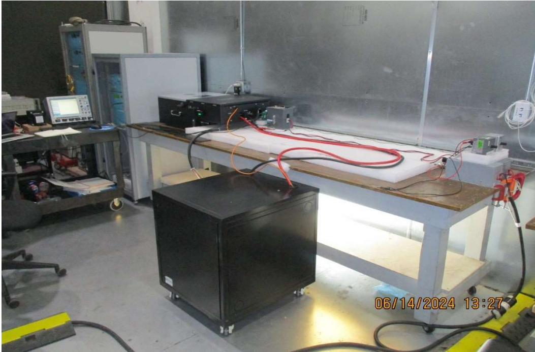
Test Setup for CS117, General Waveform #2 & #3 Test Setup for Inverter
