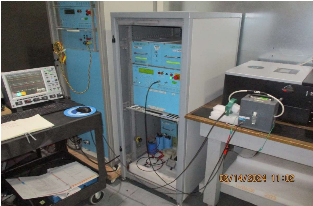
General Test Setup for CS117, General Test Setup for Waveform #3 – Short Circuit
