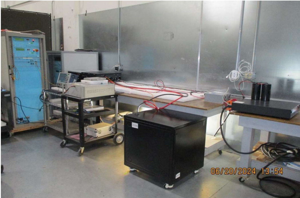
Test Setup for CS117, General Waveform #1 Test Setup for Inverter
