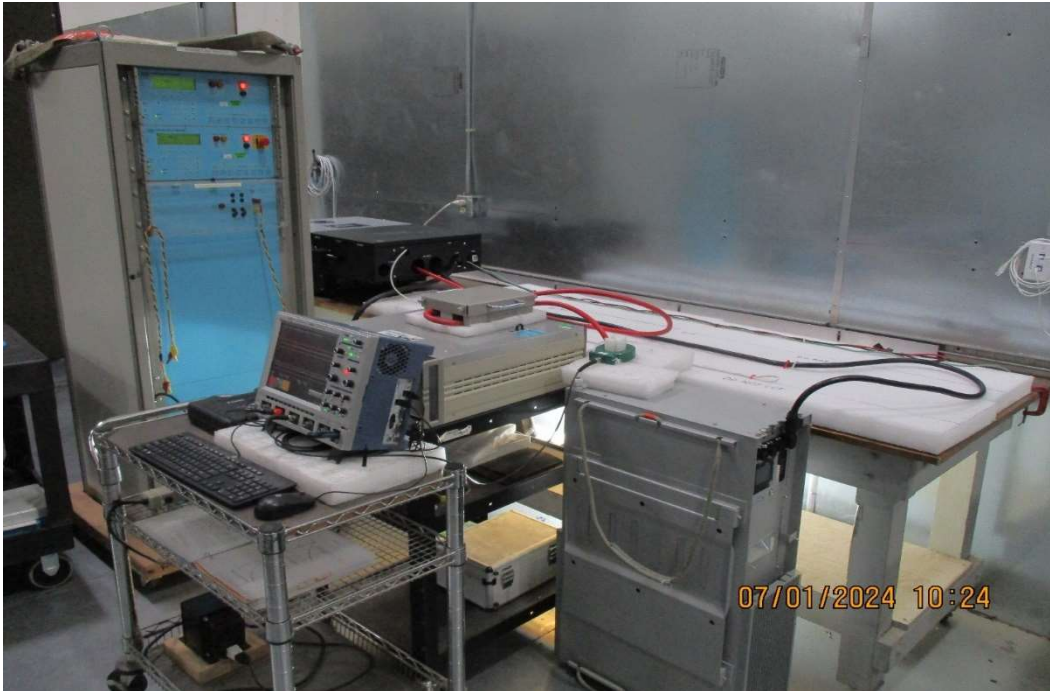
Test Setup for CS117, General Waveform #1 Test Setup for Battery Wall Mount
