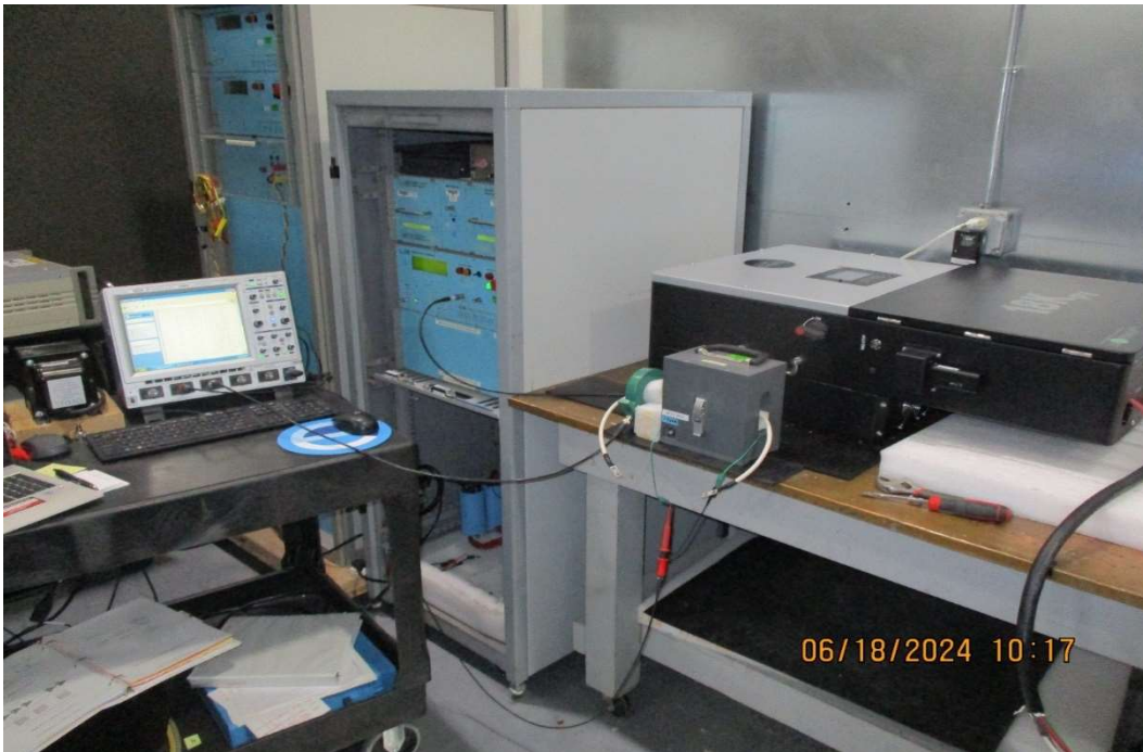
General Test Setup for CS117, General Test Setup for Waveform #3
