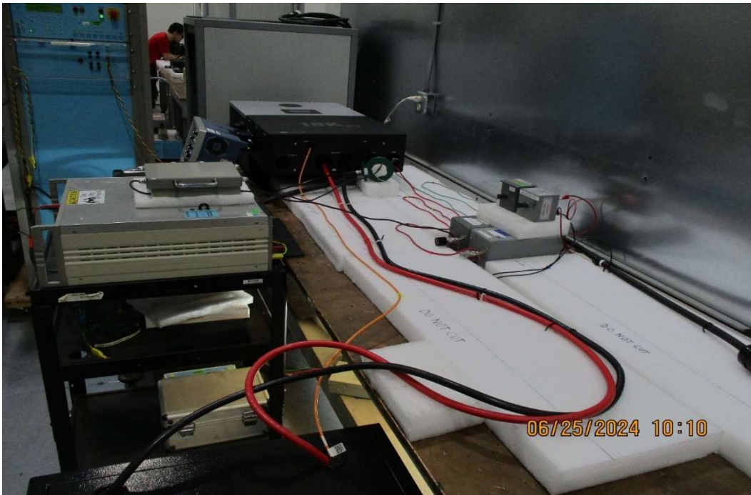
Test Setup for CS117, Actual Test Waveform #1 on AC Line 2
