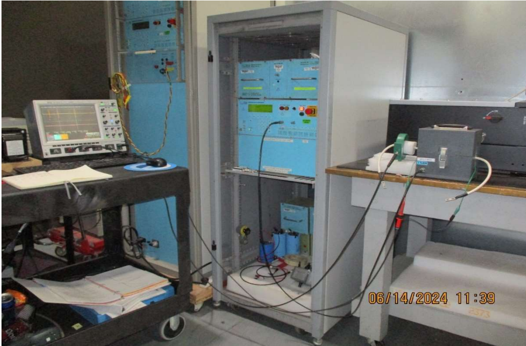
General Test Setup for CS117, General Test Setup for Waveform #3 – Open Circuit
