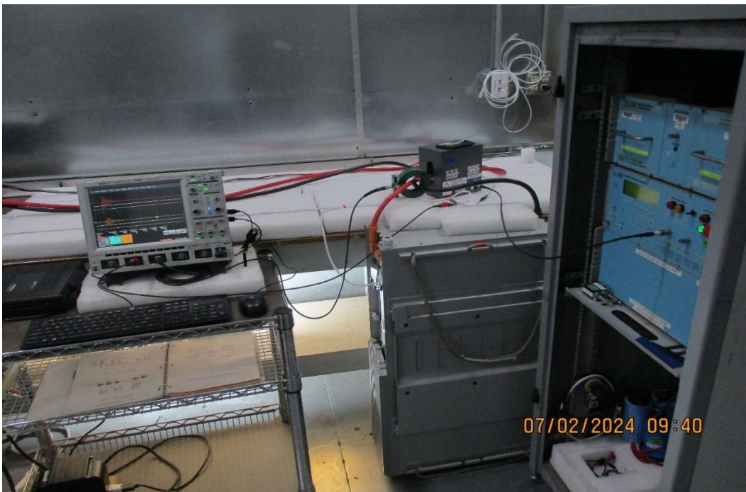
Test Setup for CS117, Actual Test Waveform #2 & #3 on Battery Bundle
