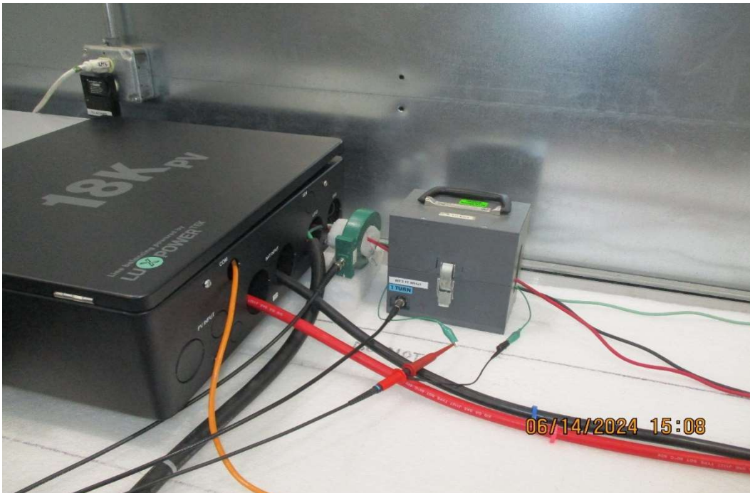
Test Setup for CS117, Actual Test Waveform #2 & #3 on AC Line 2
