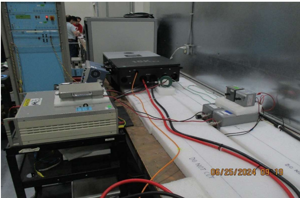
Test Setup for CS117, Actual Test Waveform #1 on AC Bundle
