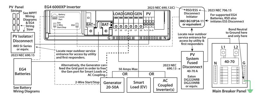
DRAWING #6000XP-V1-1L-1, VERSION 1.2 ©2024 EG4 ELECTRONICS, LLC. ALL RIGHTS RESERVED. THIS DIAGRAM IS FOR ILLUSTRATIVE PURPOSES ONLY. EG4™ IS NOT RESPONSIBLE FOR ACCURACY. FINAL WIRING DIAGRAMS SHOULD BE
