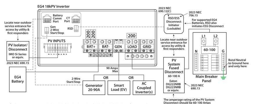
The inverter can accept BOTH DC-COUPLED AND AC-COUPLED SOLAR at the same time.
