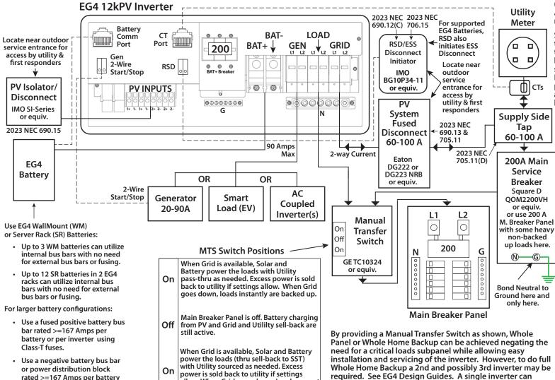
UPPLY SIDE TAPS - If your Service Entrance has a 200 A rated Main Panel bus and a 200 A Main Breaker, a 40 A Backfed Breaker can be used (see Backfed Breaker diagram). Alternatively, a Supply-Side Tap may be used.
