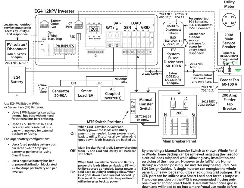
FEEDER TAPS ARE THE IDEAL AND SAFEST WAY TO TIE YOUR INVERTER TO THE UTILITY GRID while achieving whole home backup, full solar backfeed, and full battery charging capability while fully protecting your home's wiring. However, Feeder Taps must be installed correctly.
