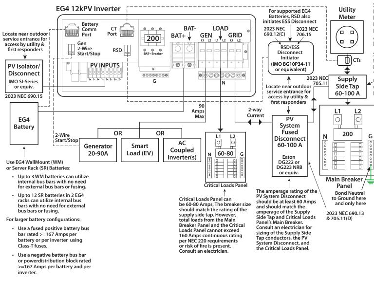
SUPPLY SIDE TAPS - If your Service Entrance has a 200 A rated Main Panel bus and a 200 A Main Breaker, a 40 A Backfed Breaker can be used (see Backfed Breaker diagram). Alternatively, a Supply-Side Tap may be used .
