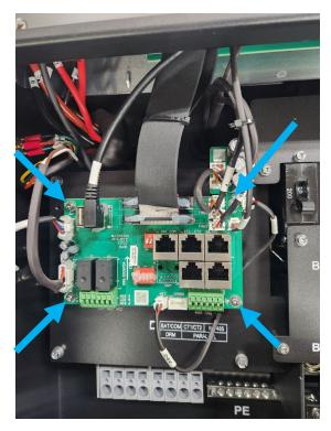
3. With the interface board out of the way, locate the rear panel and remove the 6 screws as shown below:
