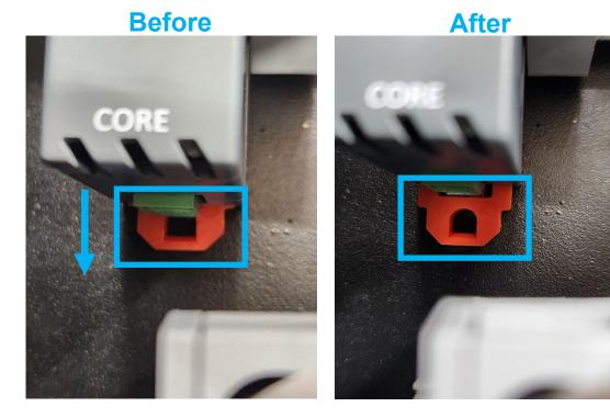
7. To complete the removal, locate the power cable on the top of the transmitter as shown below and unplug.
