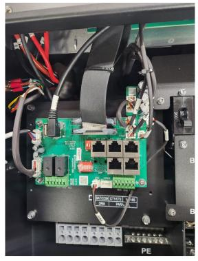
2. Remove the 4 screws shown below, then move the interface board out of the way.
