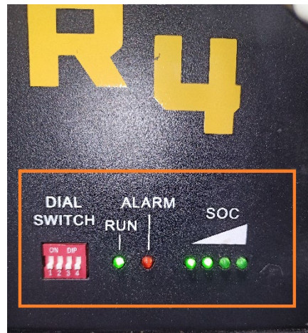
LifePower4 LED Status after successful update
