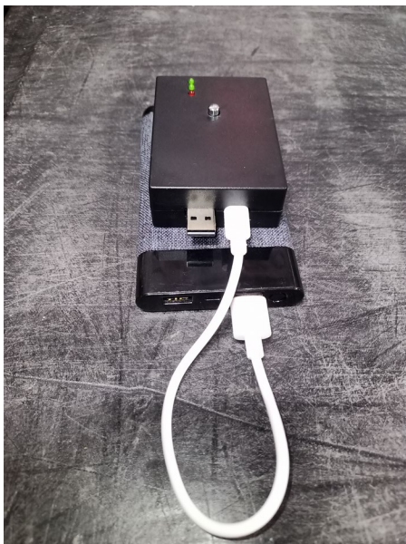
Dongle being powered by a mobile power bank
