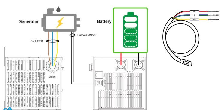
NOTE: The Chargeverter-GC comes built-in with a cooldown period when using a generator to charge. This function activates once the batter preacties the set 30C/Voltage stop point which allows the generator ~2 minutes to cooldown.
