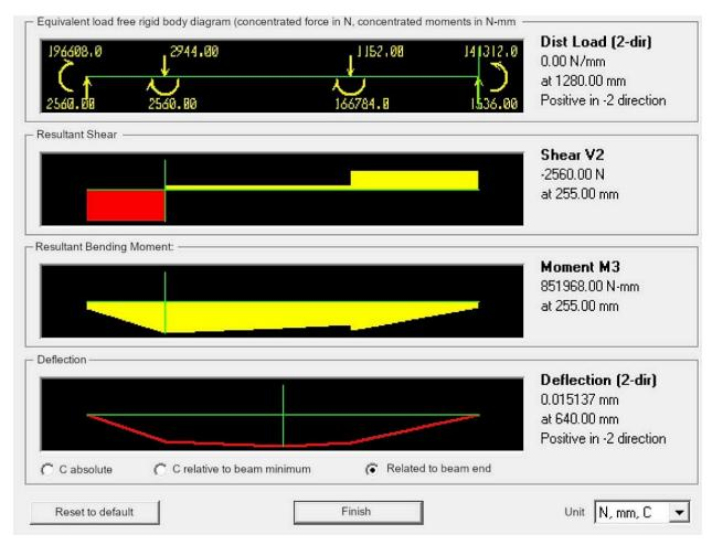
${\rm M}_{max}$  = 851968 Nm------- Max Moment  $\sigma_{max} = \frac{{\rm M}_{max}}{{\rm W}_{y1}} ------ {\rm Max Stress}$   $\sigma_{max}$  = 240 MPa------ Does not exceed max load capacity
