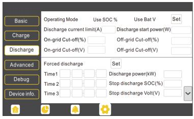
When the inverter detects the import power is higher than this value, the battery starts discharging; otherwise, the battery will stay in standby.
