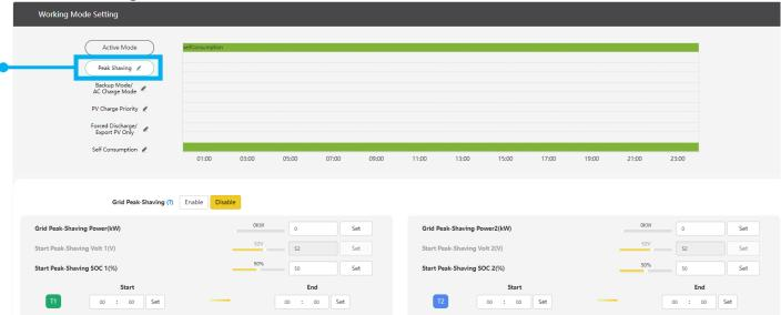
When setting the station into this mode, the inverter will use peak-shaving to avoid peak demand charges from the grid. The user will be able to configure the system to pull limited (or no) power from the grid for charging batteries or powering loads by setting maximum power in kW, according to SOC/voltage, and by setting time of use.
