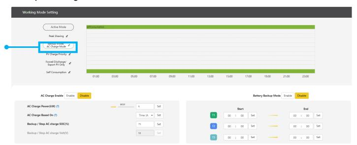
When setting the station into Backup/AC Charge mode, the user can configure the system to prioritize charging batteries from grid power. The user can configure to charge with grid based on maximum power in kW, SOC/voltage, and by setting times of use.
