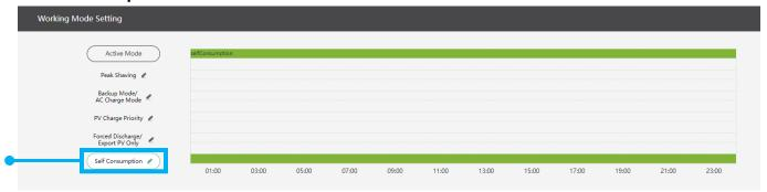
The station will default to Self-Consumption mode. The order of priority for powering loads is Solar > Battery > Grid. The order priority for solar power is Load > Battery > Grid which creates an ideal scenario when needing to prioritize solar power generation over other types of power.
