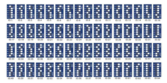
ID code bits correspond to binary digits, right side represents "ON", left side represents "OFF". The up (or right) of the code bit is the low bit, and the down (or left) is the high bit. The code range is 0~63, and the communication mode can support up to 64 modules in parallel. **Note** - If your battery contains 4 dip switches, the code range is 0-15, and the communication mode can support up to 16 modules in parallel.
