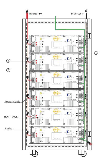
In the above figure, there are 6 EG4-LL 24V 200Ah batteries wired in parallel. This battery bank still maintains the appropriate 24V needed for Inverter/Charger systems. However, the Amp hour rating of this bank has increased to 1200Ah.
