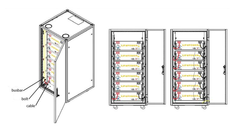
In the above figures, there are 6 EG4 Lifepower4 24V 200Ah batteries wired in parallel. This battery bank still maintains the appropriate 24V needed for most Inverter/Charger systems. However, the Amp hour rating of this bank has increased to 1200Ah.
